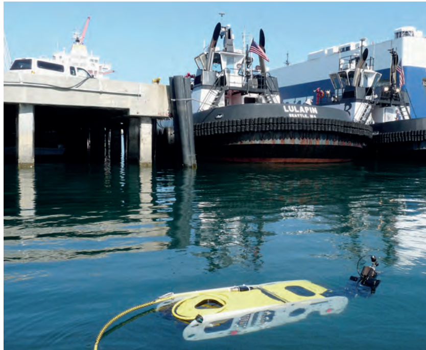
Pictured: Saab's Sea Wasp ROV at Hueneme Port, California, during Coastal Trident exercise in 2016. Sea Wasp can also operate upright to enable observation of a quay or the side of a ship. Photo: Saab Seaeeye
