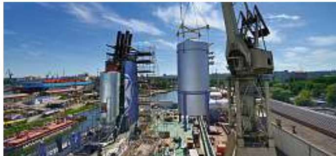
A DFDS vessel is installed with an Alfa Laval scrubber
