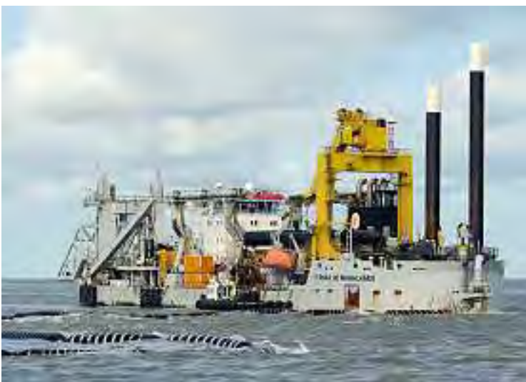
Working nearshore, self-propelled CSD Fernão de Magalhães pumps sand to the shore
