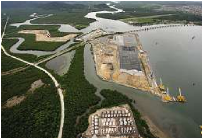
The sediment-filled geotubes can be seen on the island
