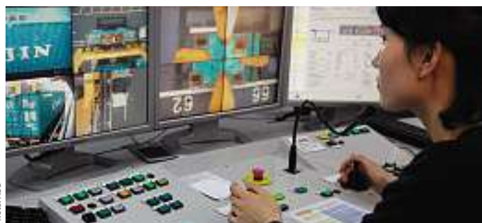
A stacking crane control room equipped with ABB's system in Korea. Crane operators can sit elsewhere in the port and control the crane remotely
