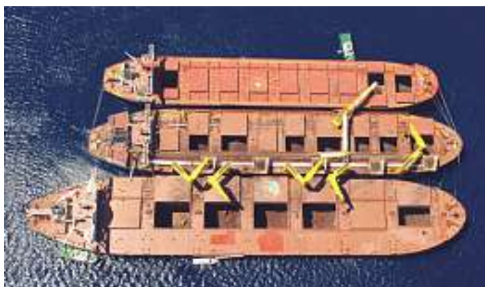
Subic Bay's Ore Fabrica transfer station (centre) transships ore from the 402,347dwt VLOC Vale Brasil (bottom) to the 179,385dwt Ore Pantanal (top)
