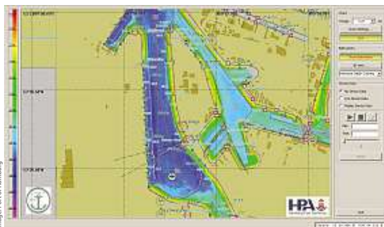
A view of Hamburg's Port ECDIS showing gridded bathymetry
