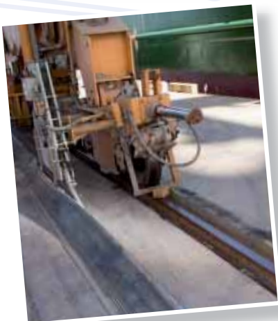
Panzerbelt is our patented cable protection system that powers shore-to-ship cranes. It incorporates a continuous semi-flexible belt, made from rubber with a steel inlay, that lies over channels cast in the quay.
