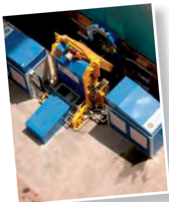
MoorMaster™ is currently in use in Australia, Canada, Denmark, New Zealand and Oman. Compared to lines, the system offers dramatic reductions in ship motion – for faster loading and unloading.
