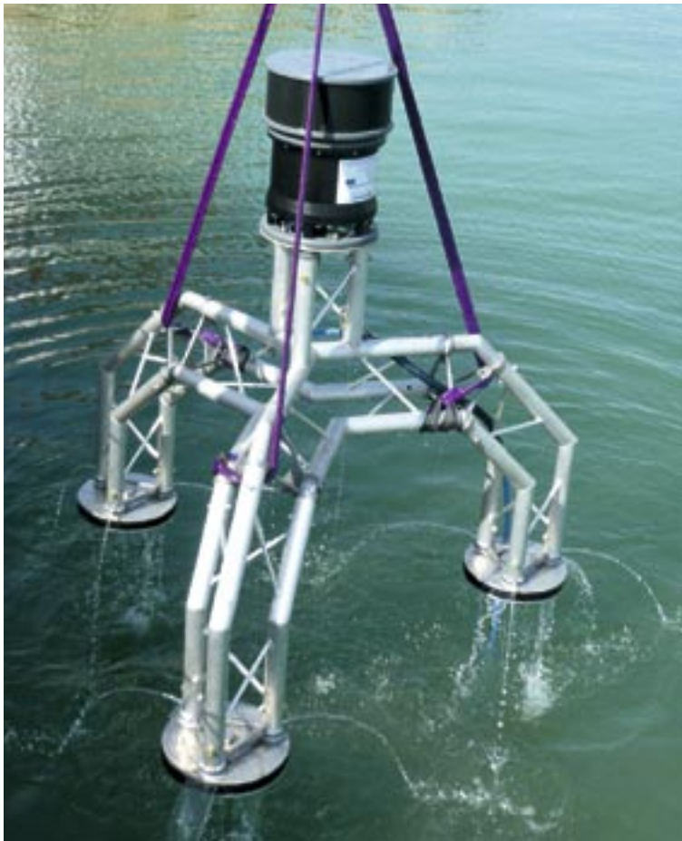
A Sentinel sonar head being deployed... it can detect and track a number of different targets
