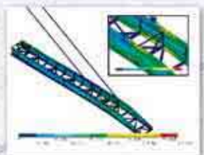
Taiwan FEM analysis to determine stress points on boom extension
