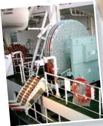
AMP can be fitted right onto the ship itself, with a single high-voltage cable, or it can be fitted inside a container that's placed on the ship, for a truly modular power source that connects to the dock or a floating barge.
