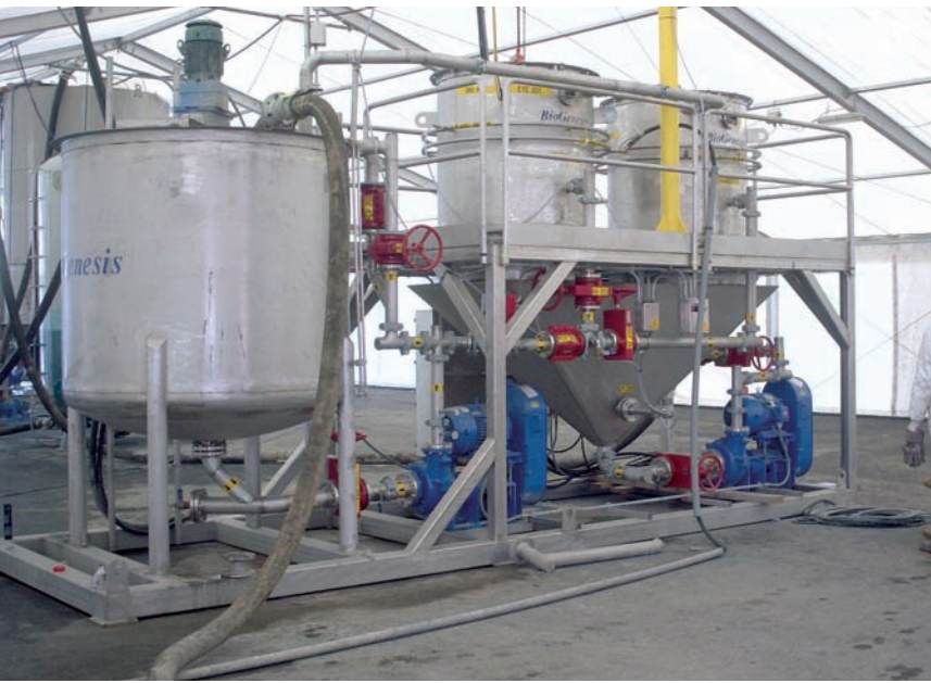
Processing the sediment (above) which was highly contaminated, but was still turned into bricks
