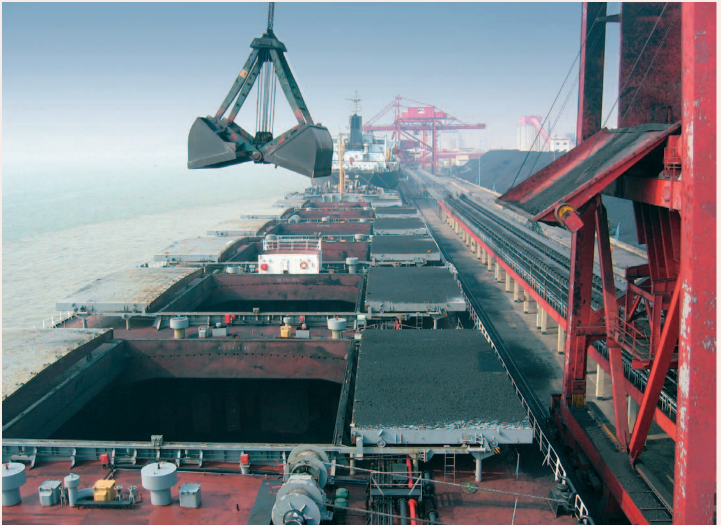
All cargo residues, like the coal on the hatch covers of this bulk carrier, are now classed as garbage
