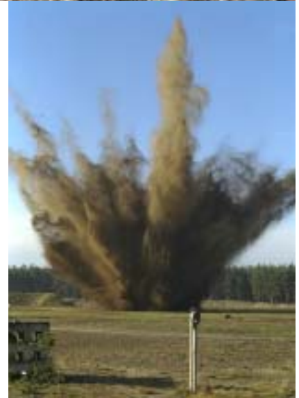
A test at the TNO laboratory of the fireworks that were involved in the explosion
