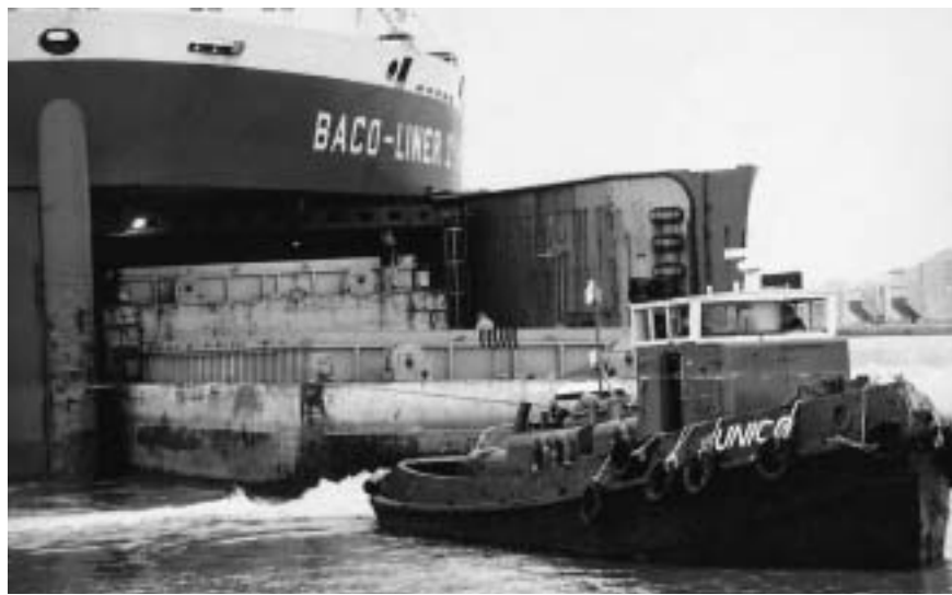
Barges are towed out of BACO Line 2 at the Port of Tilbury
