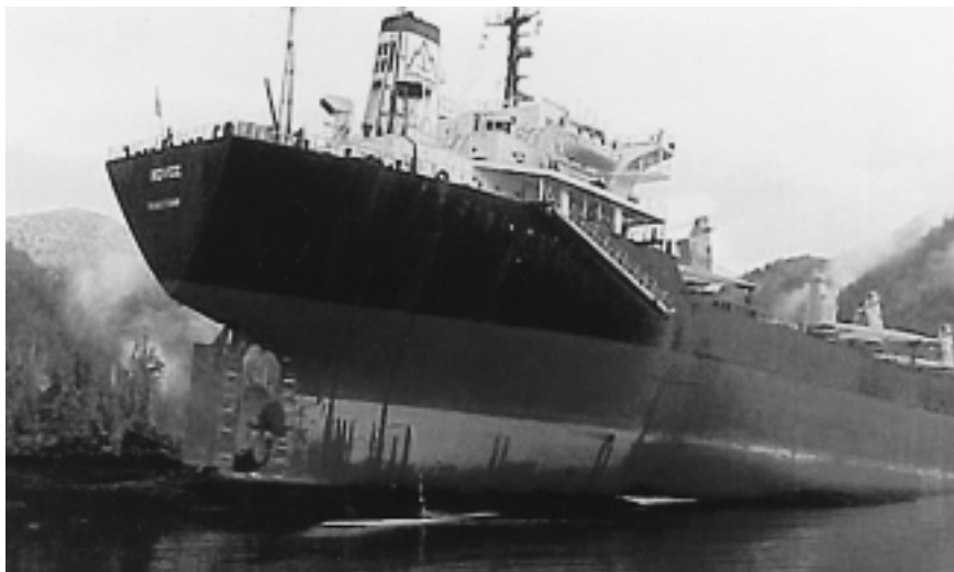
The 35,000 dwt OBO Bovec went aground near Prince Rupert, British Columbia, in March 2000. The vessel was in ballast. ISU salvors removed fuel oil prior to a successful refloating.
