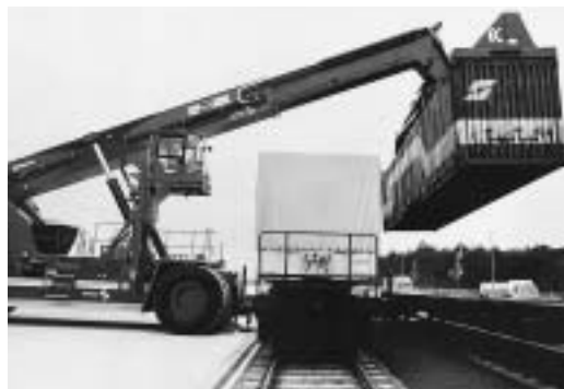
The second-rail capability of the ContChamp is clearly demonstrated in this view of operations at ÖBB's Terminal
