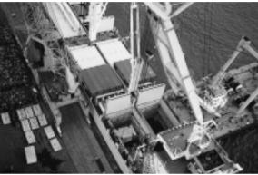
The port of Antwerp has the necessary handling equipment for all kinds of cargo. The floating derrick Brabo (photo) has a lifting capacity of 800 tonnes and is frequently used for project cargo.
