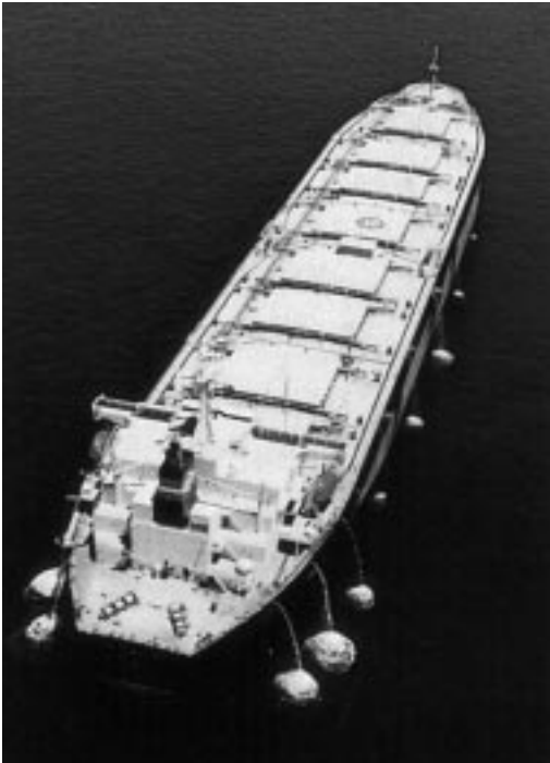
A bulk carrier discharging ballast water. Ballast water taken up in one part of the globe and discharged in another may introduce non-indigenous species which could harm the local ecosystem. (Photograph by Steve Raaymakers)
