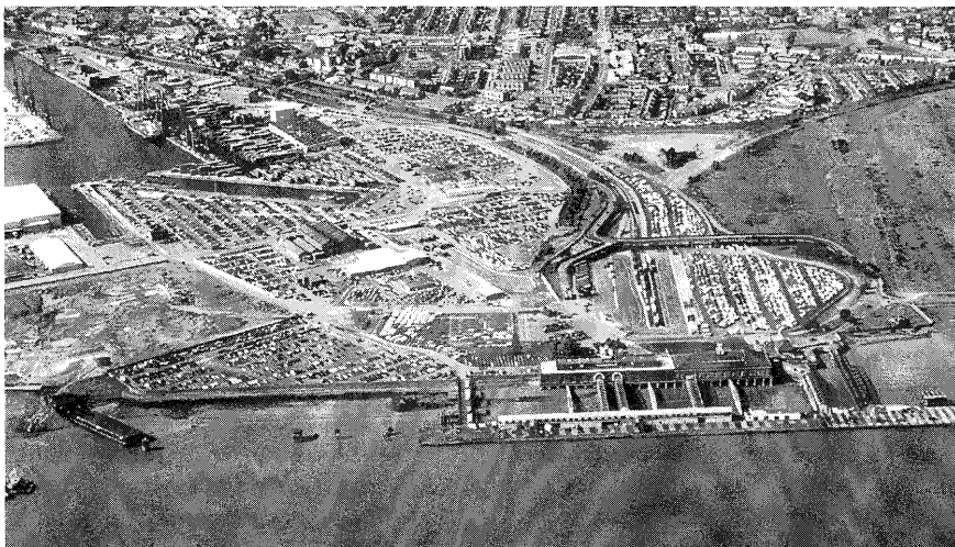
A recent aerial shot of the Port of Tilbury showing the area in the foreground, alongside the Landing Stage, where the new riverside berth is being built - and with reclamation work going on behind at the Tidal Basin
