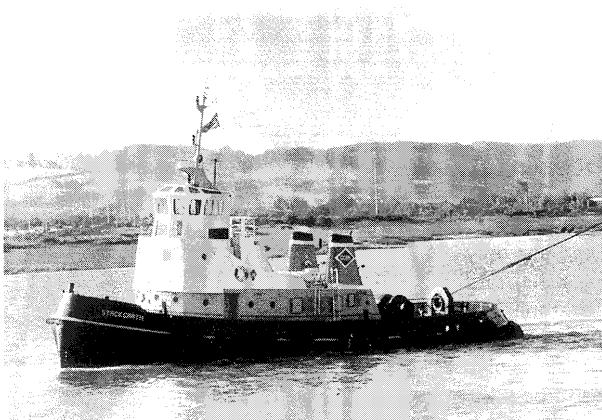
Cory Towage's tractor tug, Stackgarth , has been transferred to the company's Bristol fleet. To suit her for her new duties, she underwent extensive modification and refurbishment at the Dunston shiprepair yard in Hull. The wheelhouse has been shortened and a new central control console installed to provide enhanced all round visibility.
