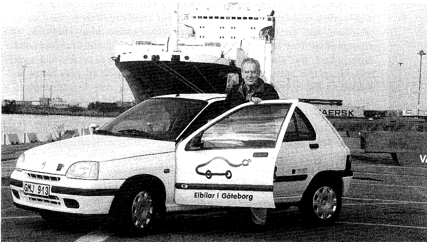
The Port of Göteborg AB is testing a battery-driven Renault Clio as a terminal car in its Älvsborg roll on/roll off harbour. For environmental reasons, the electric car has an advantage, not least on the cargo decks inside roll on/roll off vessels. Also, the limitations of battery-operated vehicles in terms of range and speed are less crucial within a port terminal.
