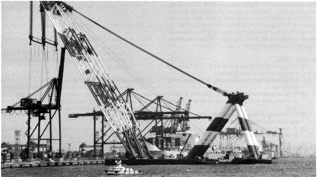
A gigantic floating crane lifts a gantry crane and puts it back on the rails after it has been repaired.
