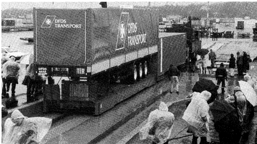
Tow platforms were used at the Alicon demonstration at the Port of Göteborg recently, one for a trailer, the other for containers. The platforms hover on four air-cushions each, the air for which is supplied by a compressor on the terminal locomotive pushing or pulling the platforms. A rail guides the train of platforms in the terminal, on the ramp and on the vessel.
