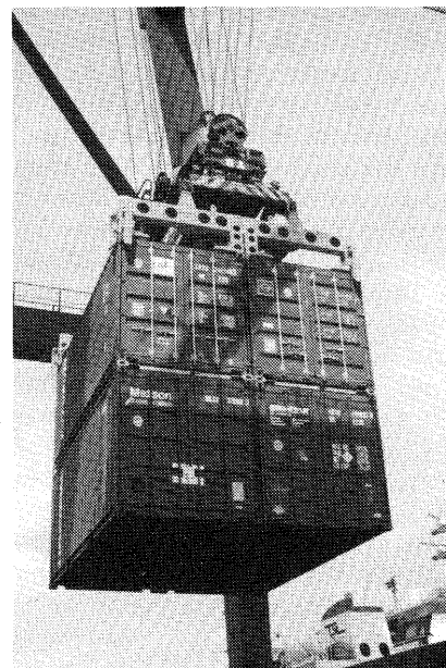
Two blocks of two vertically connected boxes under the newly designed spreader being hoisted
