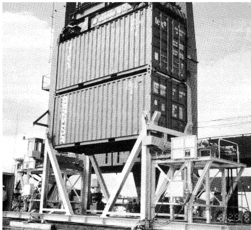
A block of two, vertically connected, being hoisted out of the block-making apparatus for loading (unloading is the reverse process of loading)
