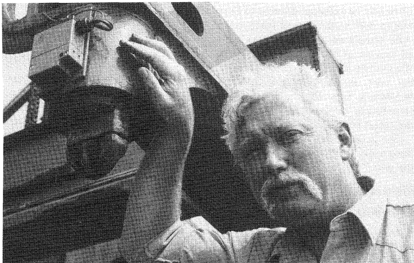
Port of Gothenburg machinery surveyor Lennart Wartig showing the location and tiny size of the box-like optical device that aligns container spreader to container on a Port of Gothenburg straddle carrier.
