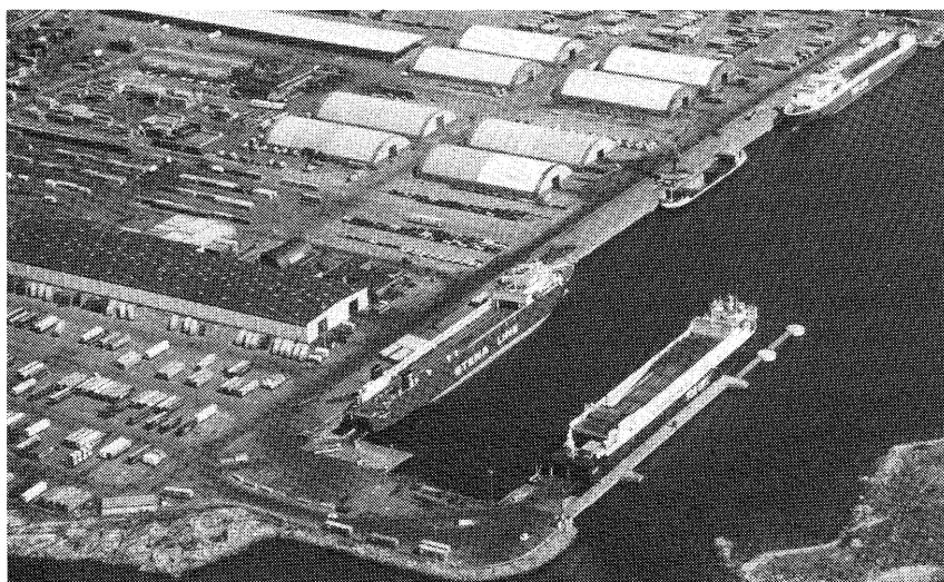
With the exception of the passenger/cargo ferries berthing in the city part of the port, most of Gothenburg's ro/ro's are to be found in the Älvsborg Harbour, dominated by the Tor Line terminal. Custom-built for ro/ro, Älvsborg is well equipped with quay ramps but lack permanent crane support.
