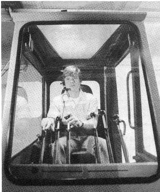
A trainee takes control of the Digitran crane simulator cab. Hydraulic actuators underneath the cab provide realistic crane motion.
