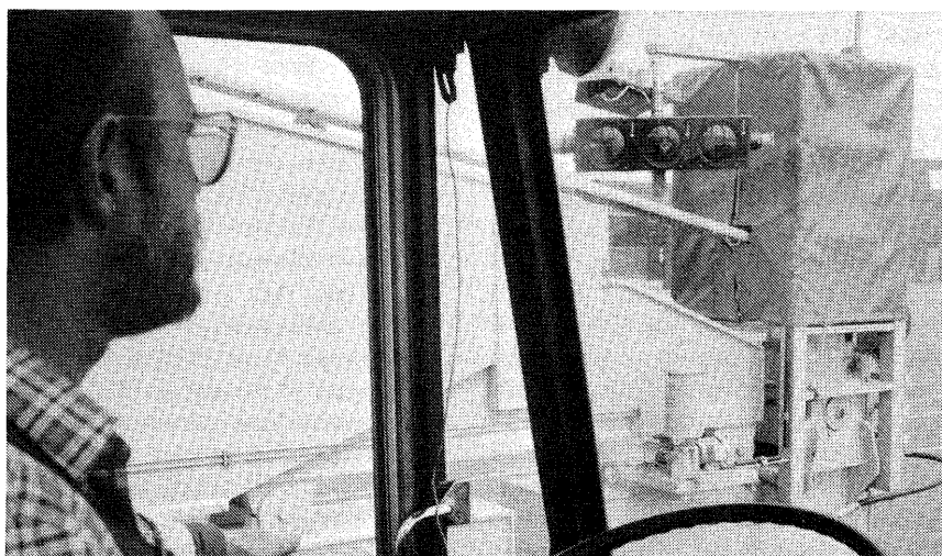
The container positioning system developed within the Port of Gothenburg works with infrared light.
