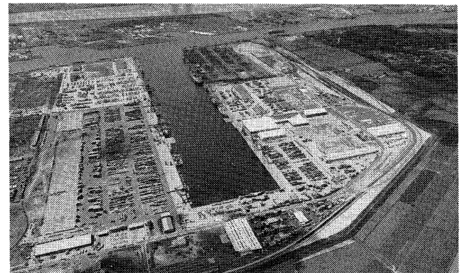
Very soon a special dock had to be built for the handling of containers: i.e. the Delwaide dock which has a quay length of 4.5 km. The depth of the land between the quaywall and the road behind it varies between 500 and 800 m.
