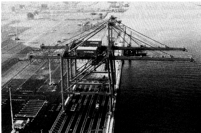
Two of the four "New Generation" Paceco Portainers recently put into operation at the Port of Seattle, Washington. The two cranes recently ordered by the port will be identical to these cranes. All six of the cranes will be capable of handling the wider "Beyond Panamax" ships currently on order.
