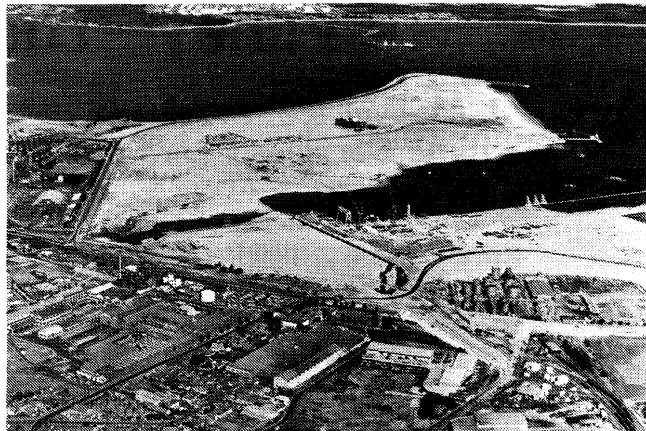
(Photograph D—Aerial view of Brotherson Dock) Two container terminals of 42 and 38 hectares are being developed along the sides of Brotherson Dock, the waterway between the two sections of reclamation.
