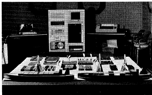
London, 12 June, 1975: —The physical model of the berth, with the computer equipment in the background, used in the National Ports Council Container Berths Simulation Analysis.
