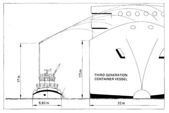
In respect of their size (about 28.5 m in length by about 9 m beam), installed propelling power ( $2 \times 1100$  hp), pulling (about 24 tons) and speed (about 22 km/hour), the new tugs will be identical to the set purchased previously, numbered from 70 to and including 76, which have been successfully operated as from 1968.
