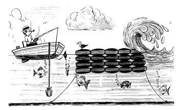
Dunkirk, N.Y., U.S.A. (Goodyear International Corporation):-WAVE BREAKERS-This cartoon illustrates how scrap tire breakwaters control the slashing power of waves. The structures are made by lashing together bundles of discarded tires with high-strength cables, ropes or plastic bands, explain Goodyear scientists who developed them.
