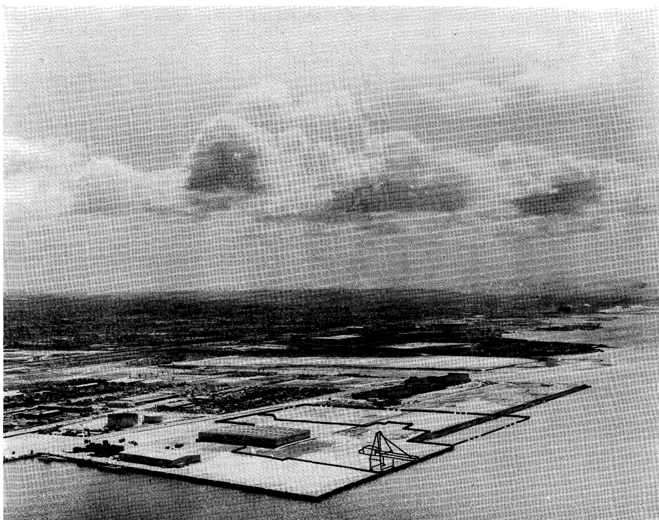
San Diego:—The National City Marine Terminal site in the South Bay. The solid line indicates the initial Container Terminal area, and the broken line the future expansion. See also diagrams on opposite pages. (Port of San Diego)
