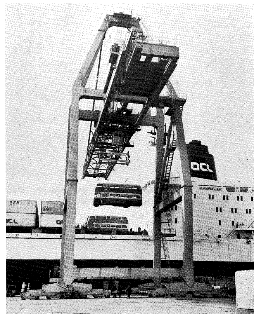
Versatile Container Crane — FACECO PORTAINER loading double decker buses in England. (Photo courtesy of the British Transport Docks Board)
