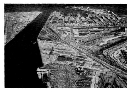
← The Middle Harbor area of the Port of Oakland includes Seatrain container terminal in foreground and new Middle Harbor Terminal behind it. When the entire area is completed, early 1973 there will be 100 acres of container terminal area and four berths served by four container cranes. Seatrain will use two berths, United States Lines will occupy another, and one berth will be a common-user facility.
