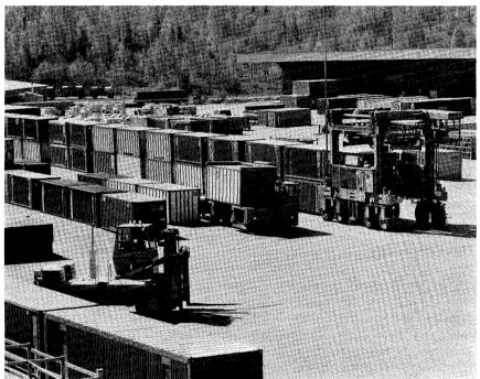
The container handling equipment includes a high-lifting straddlecarrier for 20-40 ft. containers, a side-loader with spreaders for 20-40 ft. containers and a large number of forklift trucks with capacities up to 30 tons.
