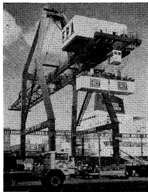
TWIN LIFT PORTAINERS serve high volume terminals
