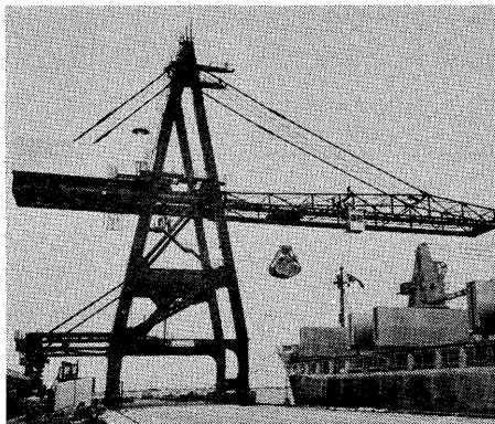
COMBINATION PORTAINERS increase utilization by handling both bulk and containers
