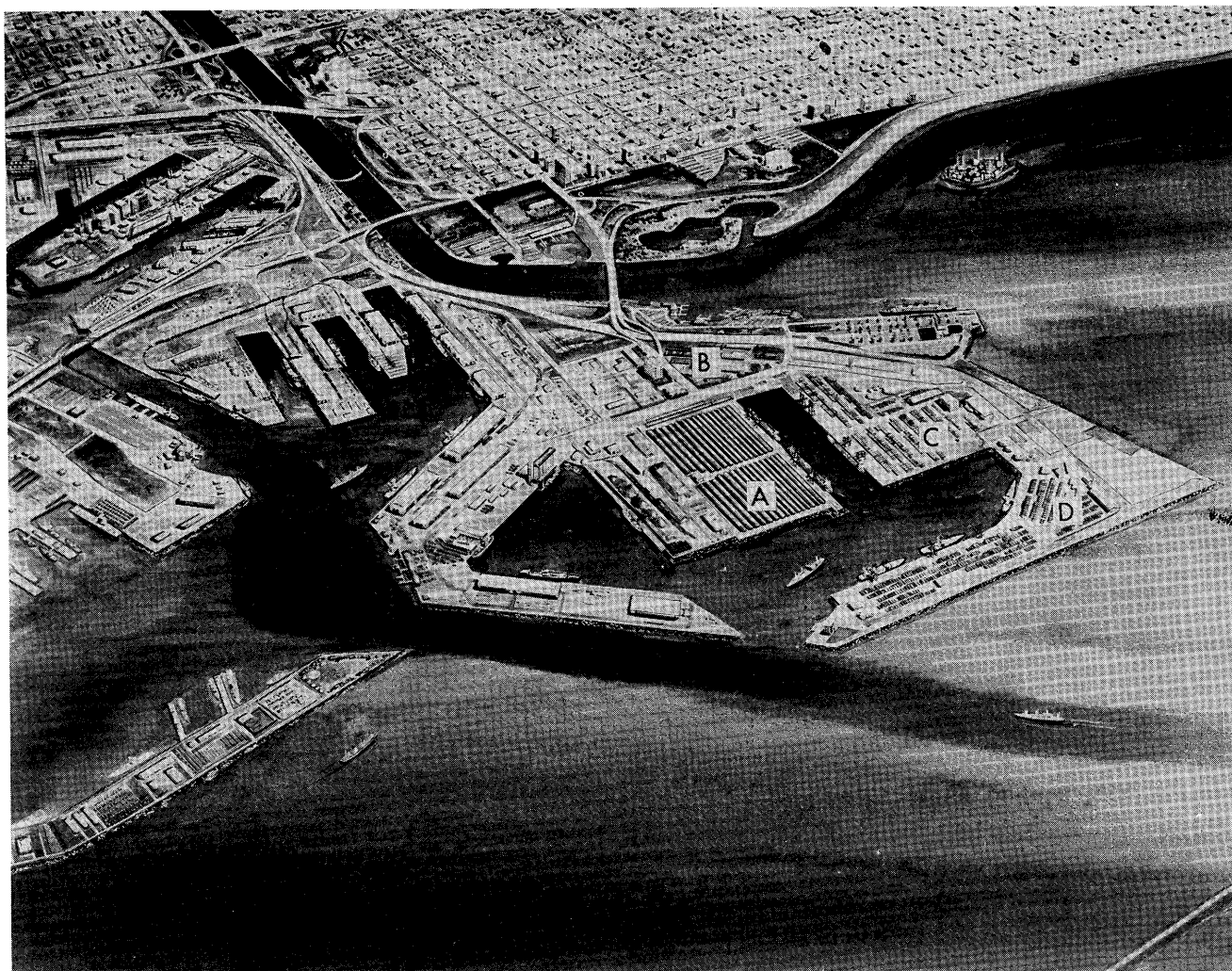
Four-part program to complete container cargo facilities within confines of South-east Basin in the Port of Long Beach is detailed in this artist's view of $30-million three-year project. Figure "A" shows the 80-acre addition for Sea-Land Service container terminal on Pier G, just south of Sea-Land's rail and truck terminal ("B") covering 16 acres on existing land. Present container terminal ("C") is being enlarged by 40 acres for Kerr Steamship Company's combined auto and container facility, while Berths 243 and 244 ("D") will be readied for container ships on 24 acres of existing Pier J. Cost of program is being met with Series A Harbor Revenue Bonds, first ever issued by The Port of Long Beach.
