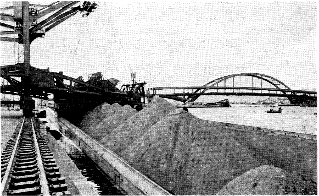
Unloader buckets rotating to unload soil from barge. (Kobe City)
