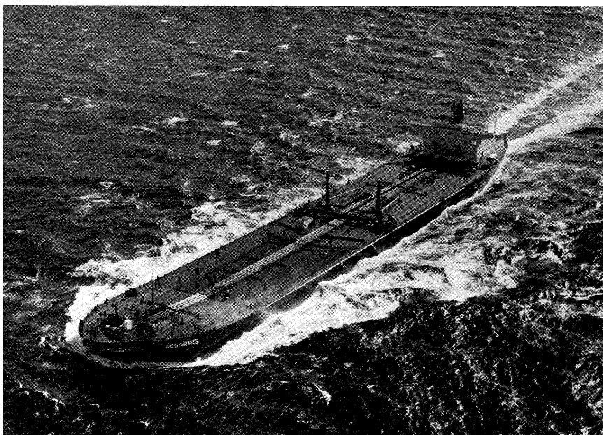
The 216,821 DWT tanker S/T "Aquarius", was completed at Sakai Shipyard of Hitachi Zosen and was delivered to the Liberian owner Cyrus Tanker Corp. on January 22, 1970. The tanker is 322.30 meters long. The main engine is a set of turbines 30,000 ps strong which yielded a maximum trial speed of 15.763 knots. The tanker is to be put into service between the Persian Gulf and the Gulf of Aqaba, and is so constructed that it would be able to pass through the Suez Canal under ballast condition when the canal is reopened.
