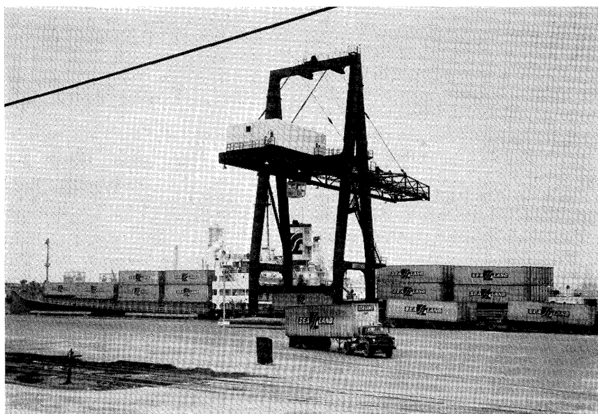
July 27, 1970:—27½ Ton PACECO Portainer, Houston, Texas. The new Port of Houston Portainer will be similar but larger than the one shown here, which was installed at the Sea-Land Terminal in 1966. (Paceco News)
