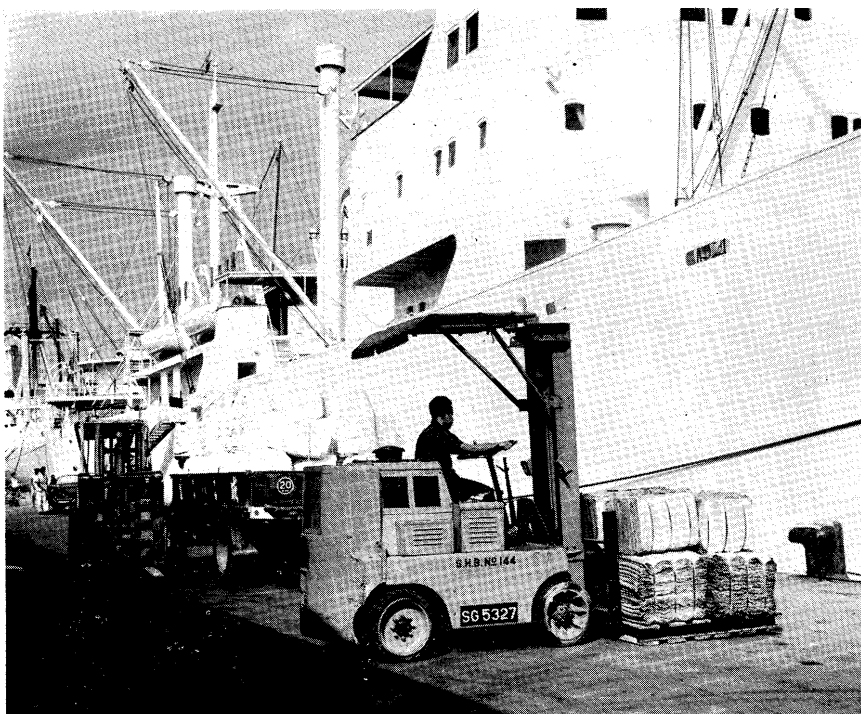
Cargo operations at the PSA wharves are carried out by the Authority's own trained labour with the aid of mechanical equipment. The Authority has over 30 mobile cranes with capacities of 2~27½ tons, over 200 forklift trucks capable of lifting up to 18,000 lbs, over 10 towing equipment up to 40 tons capacity and over 142 trailers up to 25 tons capacity.—The Port of Singapore Authority
