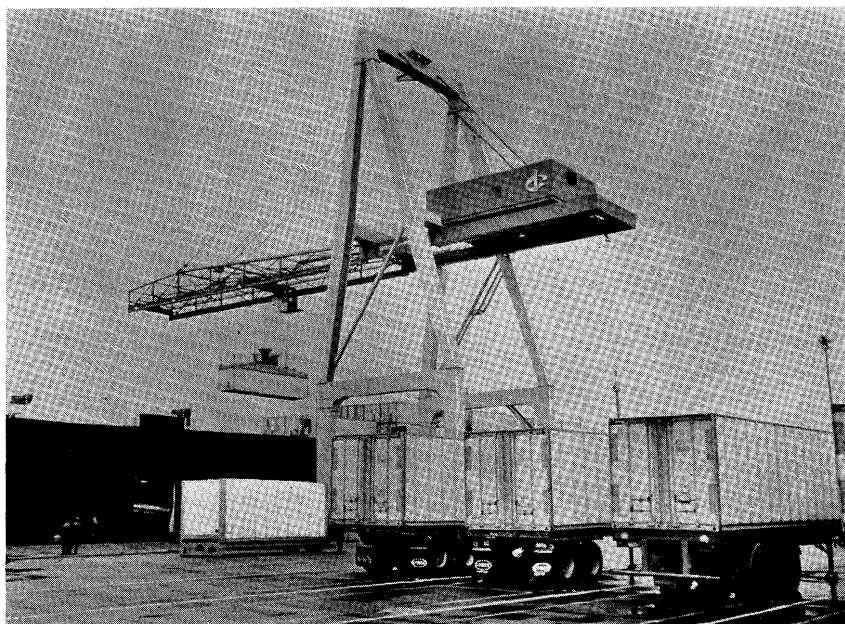
ROLL-ON/LIFT-ON —Shown being loaded during its first call at the Port of Gothenburg, Sweden, is the Atlantic Container Line's MV Atlantic Song —one of the consortium's four unique roll-on, roll-off/lift-on, lift-off trans-atlantic containerships. The vessels employ the concept of both vertical and horizontal loading and off-loading. Accomplishing the vertical (lift-on) loading is the port's new Paceco Portainer. The 27.5-ton capacity dockside crane has an outreach of 113.5 ft. and a backreach of nearly 28 ft. The Portainers are installed or under construction in five of ACL's seven ports of call in Europe and the United States.
