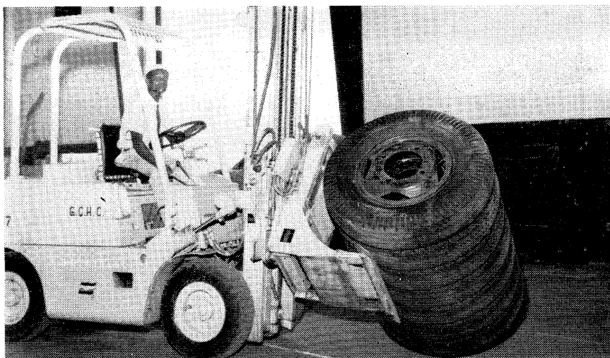
Clark D.C.Y. 50 forklift fitted with rotating reel clamp—for handling newsprint and bundles of tyres.—Tema
