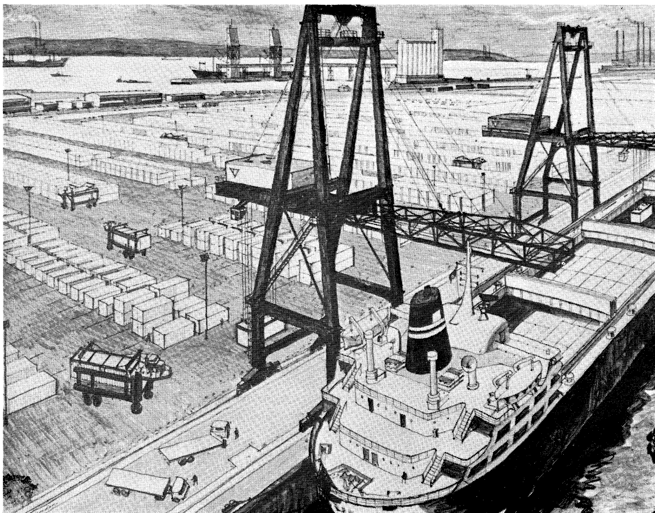
Figure 1.—Tilbury Docks. An artist's impression of a container berth. The first of several such berths will be commissioned early in 1968. The special gantry quay cranes and straddle carriers are illustrated. In the background is the new bulk grain terminal on which work has now commenced.
