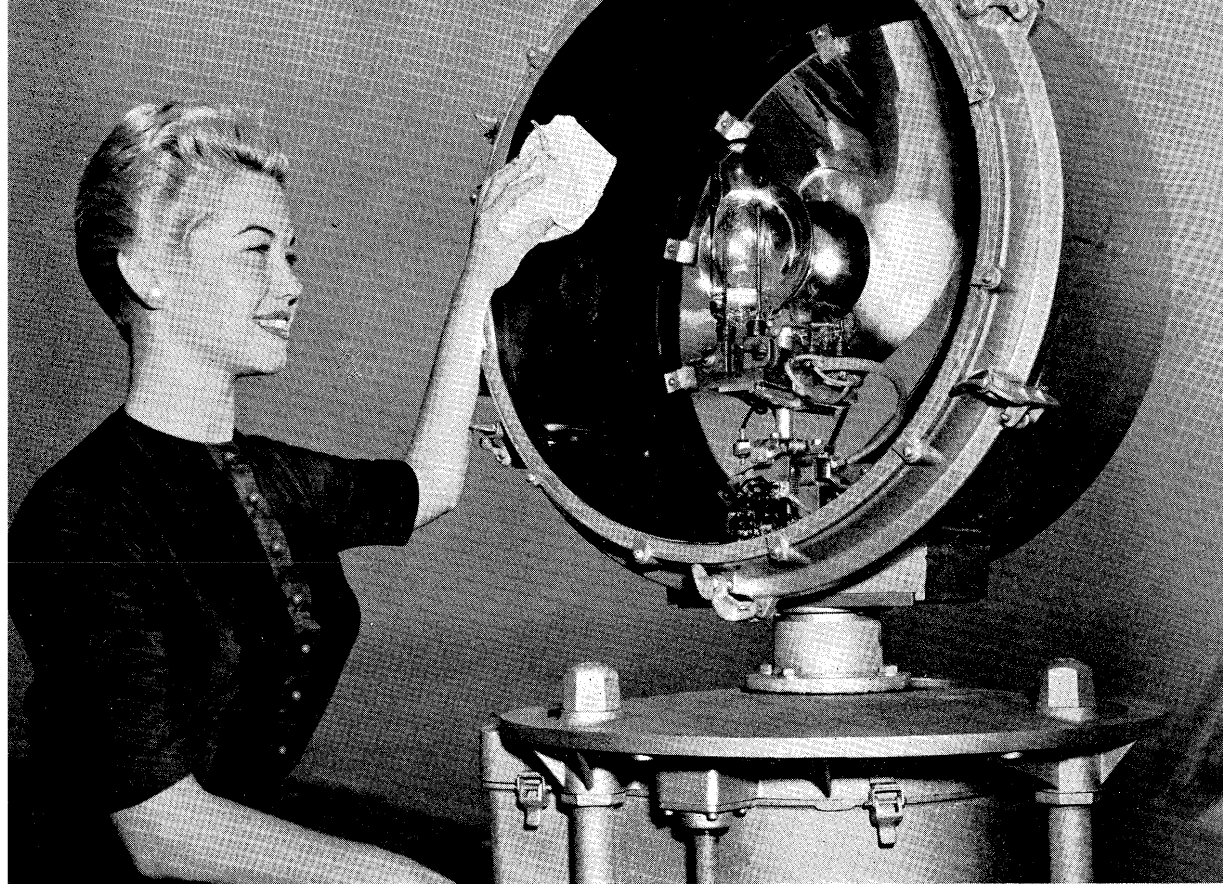
Miss Barbara Ware, of the Port of Long Beach, shines up the new beacon light located on top of the Harbor Department Administration Building. The 3,300,000-candlepower revolving light can be seen 50 miles at sea.
