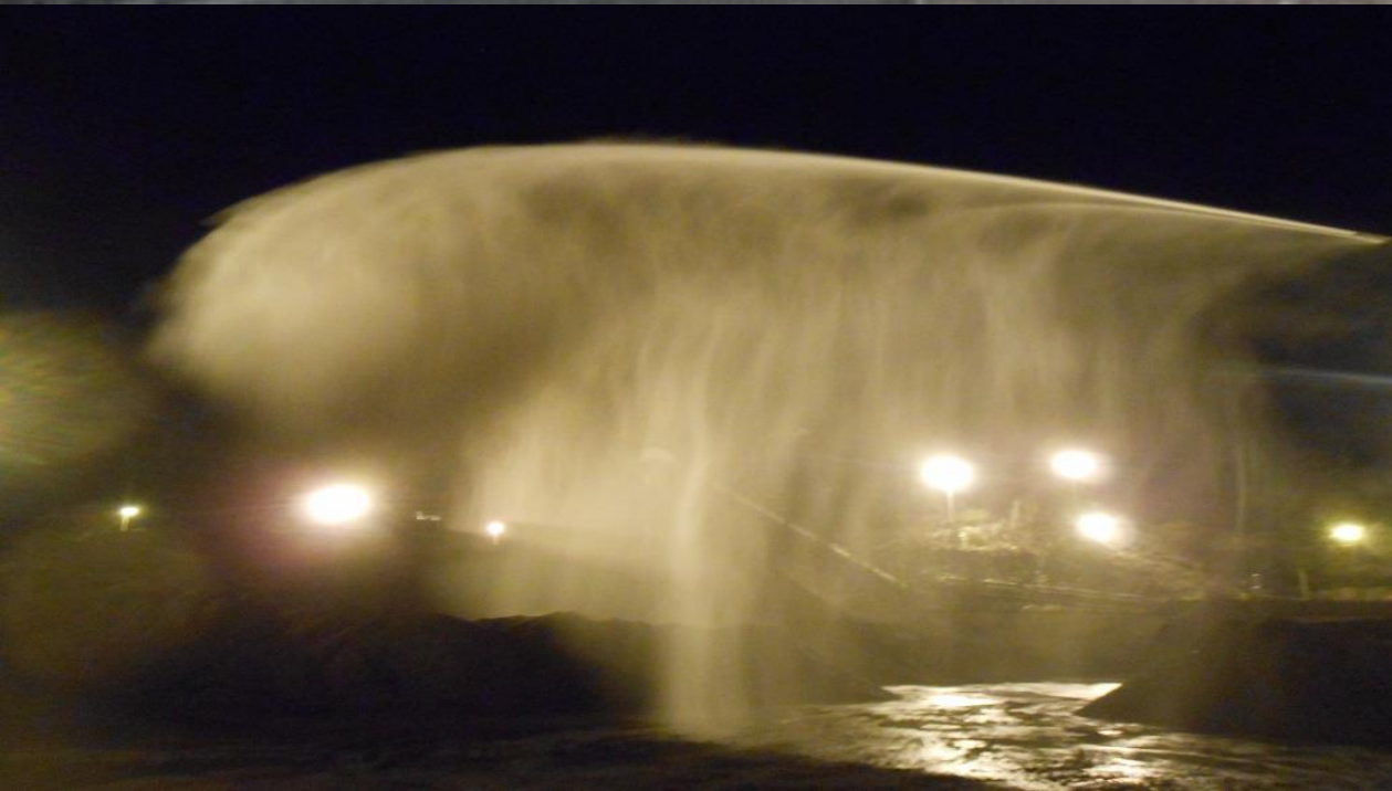
Constant humidification of exposed surfaces, with recirculating water. It increases the forces of cohesion versus aerodynamic forces.
