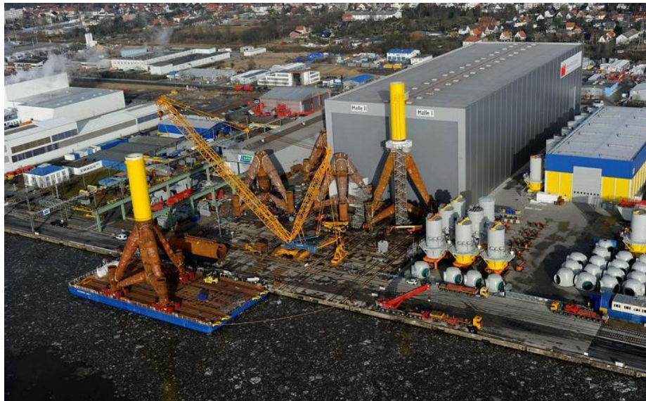
Figure 51 Pontoon-supported Transport of OWEF Foundations in the Port of Bremerhaven
