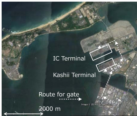
Figure 13 Trailer's routes to the terminal gates in Hakata port
