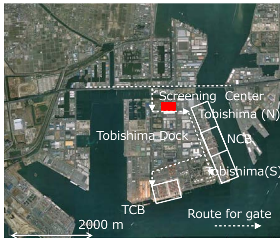
Figure 14 Trailer's routes to four container terminals and the SCS in Tobishima Dock, Nagoya port
